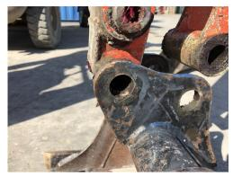
6. Lower boom to line up holes, making small adjustments as necessary
