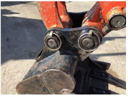
10. Slide bucket pin in, wiggling bucket if necessary and fit lynch pin
