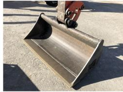
1. Rest the bucket lightly on level ground (to avoid putting pressure on the bucket pins)
