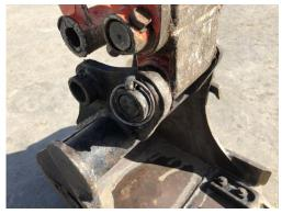
7. Slide bucket pin in by hand (it should slide in easily, no hammering) and fit lynch pin. (Note: some buckets have lynch pin locators on opposite side)
