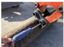
3. Push bucket pins out with large screwdriver (do not hit with hammer). If they don't slide easily reduce pressure from arm. Don't allow removed bucket pins to collect dirt or grit.
